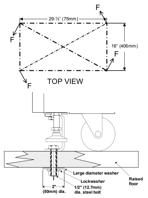
NOTE: Combination of floor material of given thickness , plus properties of large diameter washer and fastener , should result in lateral load capability to withstand shear due to load F =1500 lb (680kg), parallel to floor .
